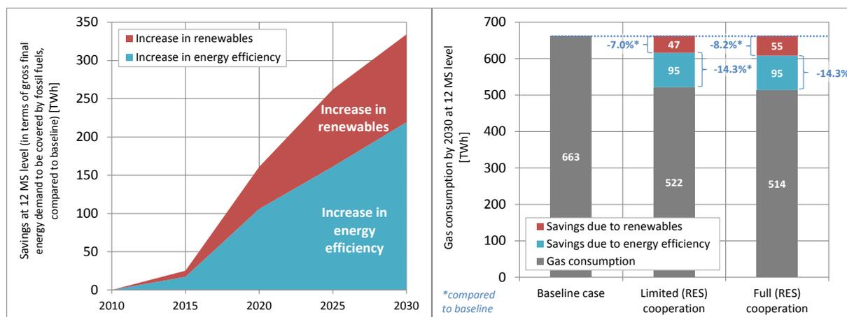
**Figure 6. Reduction of fossil energy (left) and gas consumption (right) under two alternative renewables and energy efficiency policy scenarios in the assessed 12 Member States**
